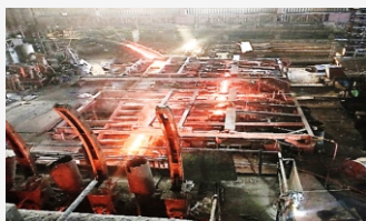
Billet Convey to Rolling Mill
